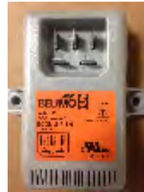
DISCONNECT TWO GREY WIRES IN FILTER SECTION OF THE RTU. THESE WIRES ARE LOCATED IN THE FACTORY WIRING BUNDLE ("PL-6"). ONE IS LABELED ENTH SENSR"AND THE OTHER IS UNLABELED. ONCE REMOVED CONNECT FEMALE ENDS TO R/A SENSOR AS SHOWN ABOVE
