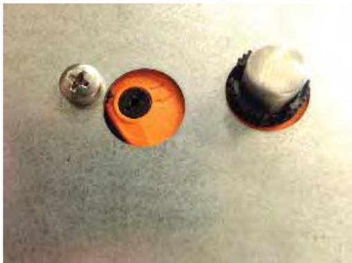
LOCATE WINDOW ON SIDE OF ACTUATOR BRACKET WHICH IS MOUNTED ON TOP OF DAMPER BLADE ASSEMBLY.
