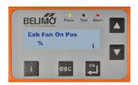
EXHAUST FAN ON POS = SET % OF ECONOMIZER O/A DAMPER OPEN THAT WILL ENERGIZE THE POWER EXHAUST
