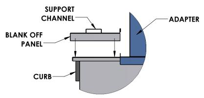
**STEP 5:** IF AN EQUIPMENT SUPPORT IS PROVIDED WITH THE ADAPTER, IT MUST BE PLACED UNDER THE SIDE THAT OVERHANGS THE EXISTING CURB. FIELD SUPPLIED SHIM MAY BE REQUIRED.
