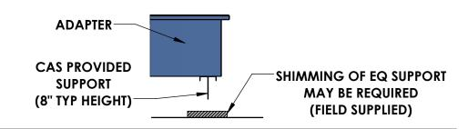
STEP 6: APPLY GASKET (PROVIDED WITH ADAPTER) TO THE TOP PERIMETER AND AIR OPENINGS OF THE ADAPTER. CAREFULLY SET THE NEW UNIT DOWN ONTO THE ADAPTER AND CHECK TO MAKE SURE IT IS FULLY SEATED.
