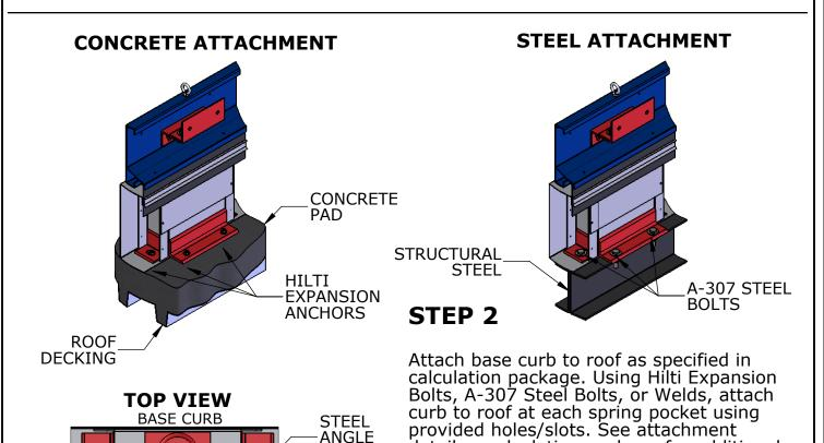
information. Ensure Curb is level and add shims under spring pockets if required.
