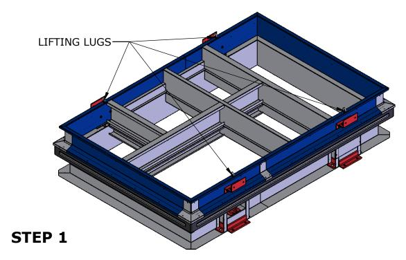
Lift isolation curb to roof using pre-existing lifting lugs. Verify location and orientation of curb as springs are determined based on unit corner weights.
