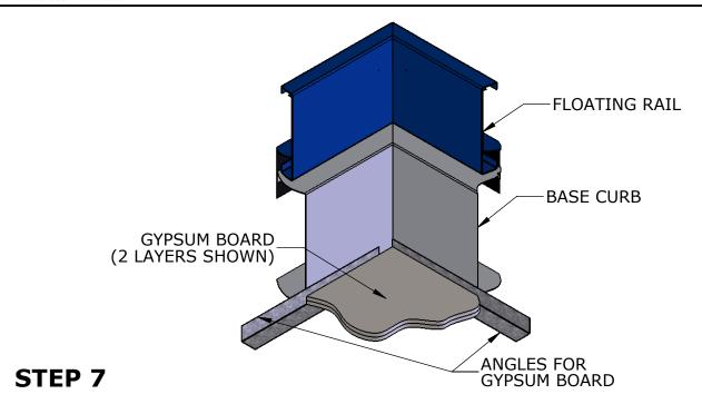
If required, install field supplied gypsum board in location specified on submittal. Place on Cambridgeport supplied angles on interior of isolation curb.
